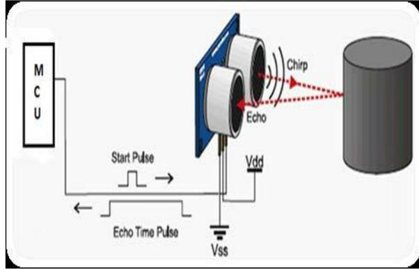
Fig 2.2 Working Principle of Ultrasonic Sensor
